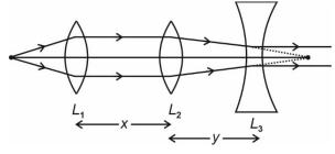
The image formed by lens  $L_2$  should be focused on second focus of lens  $L_3$ .
